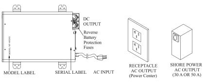
If the reverse polarity fuses are blown, it means the RV battery was accidentally connected in reverse, either at the battery or at the converter. Reconnect properly, then replace the fuse with the same type and amp rating as the original "Littelfuse" Type 257 automotive-style fuse.
